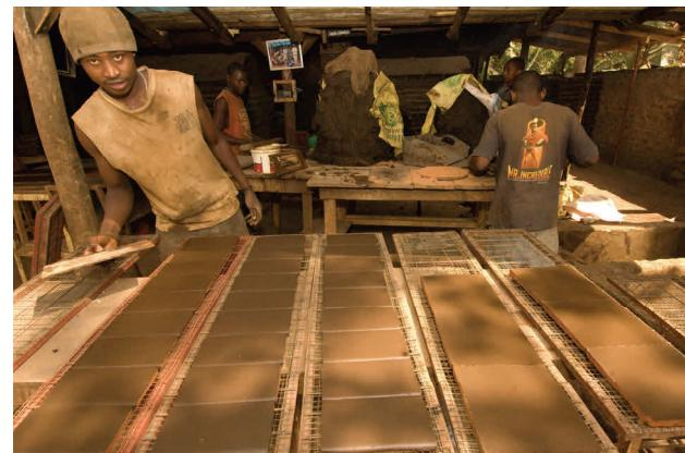
Rinse abundantly with water and a bit of a scrub during the first 1 or 2 weeks. This step is essential in removing cement residue.
